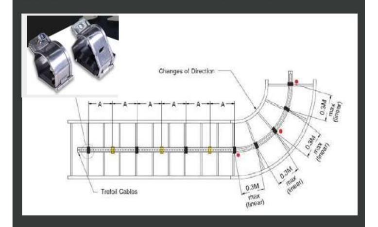
It is important that the cleats are installed properly to secure your cables:
